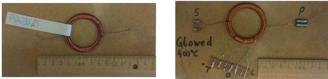
Figure C.1: Standard sample for hysteresis measurement (left) and one with a magnetostriction set-up (right)
