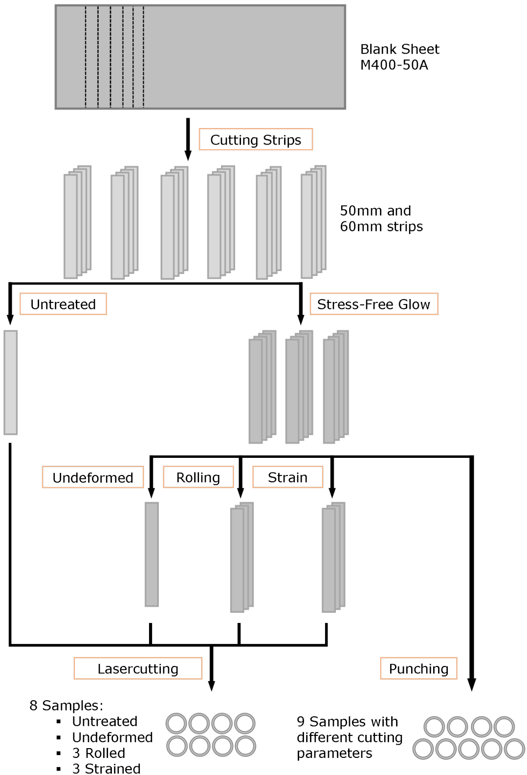
Figure 3.1: The workflow of the ring shaped samples, from the blank sheet over the different deformation processes to the rings
