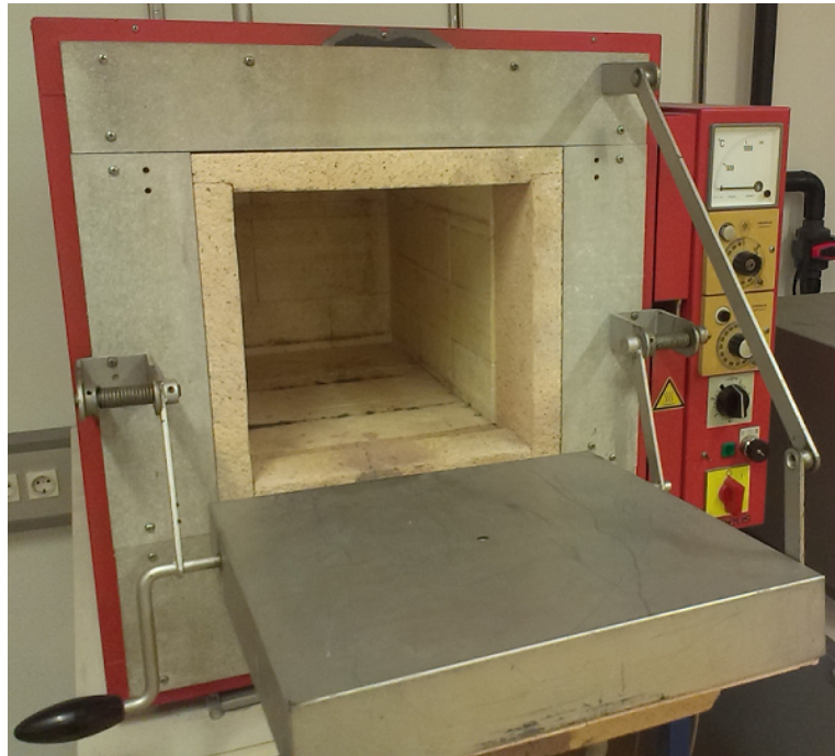
Figure 3.2: The Hareaus M1100 laboratory oven to stress-free glow the metal stripes
