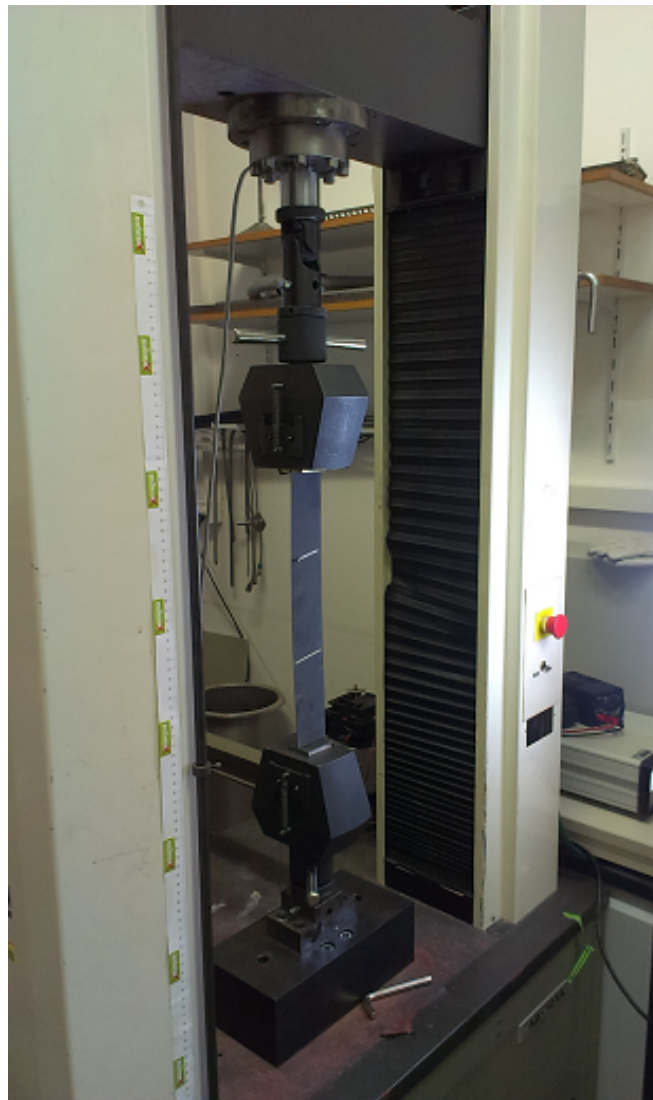
Figure B.1: Tensile machine with a M400-50A strip clamped
