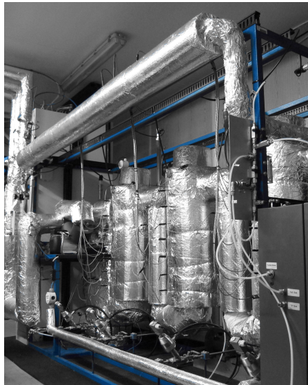
Figure 3: Picture of the WGS unit employed for fixed bed catalysis of the WGS reaction in wood gas.
