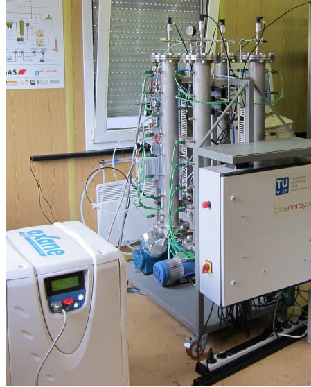
Figure 4: Right: PSA unit employed for H 2 purification in the preconditioned wood gas; Left: PEM fuel cell for the demonstration of the quality of the generated BioH 2 .
