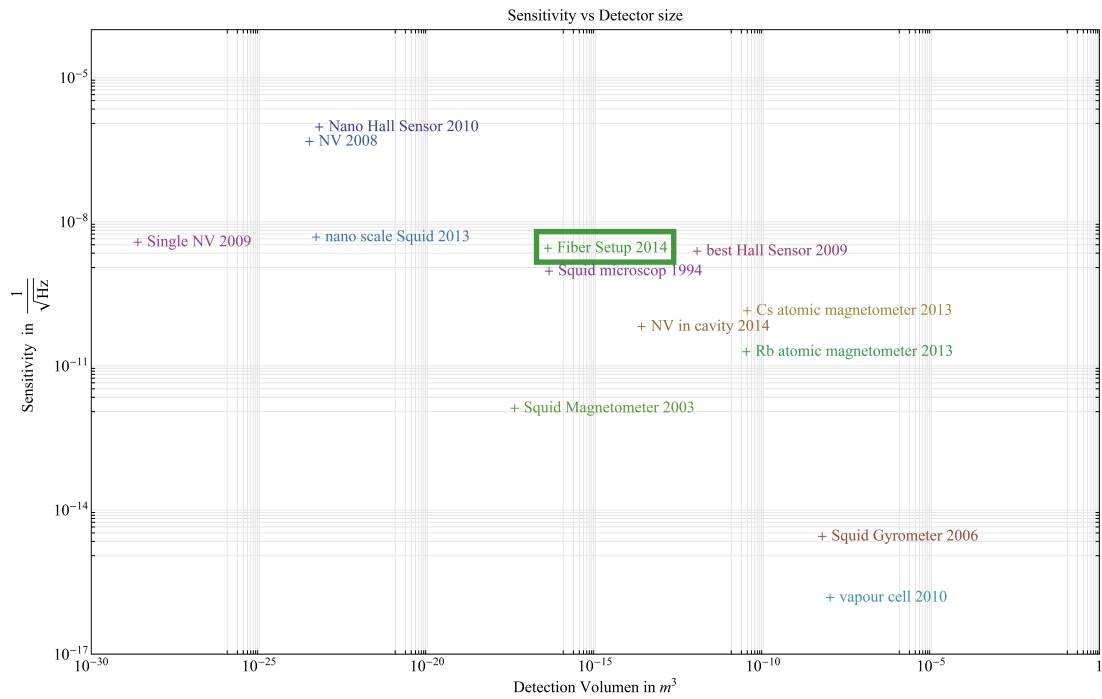
Figure 4.12: Nano Hall Sensor [11], NV [17], Single NV [2], nano scale Squid [24], best Hall Sensor [10], Squid microscope [15], Cs atomic magnetometer [16], Rb atomic magnetometer [23], NV cavity [14], Squid magnetometer [4], vapour cell [21], Squid Gyrometer [9]. The theoretical performance of our setup is framed.
