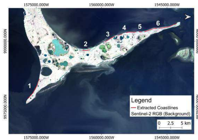
FIGURE 5.26: Bykovsky Peninsula shorelines extracted from PALSAR and PALSAR-2 data with the 6 areas marked. The background is a Sentinel-2 RGB image.
