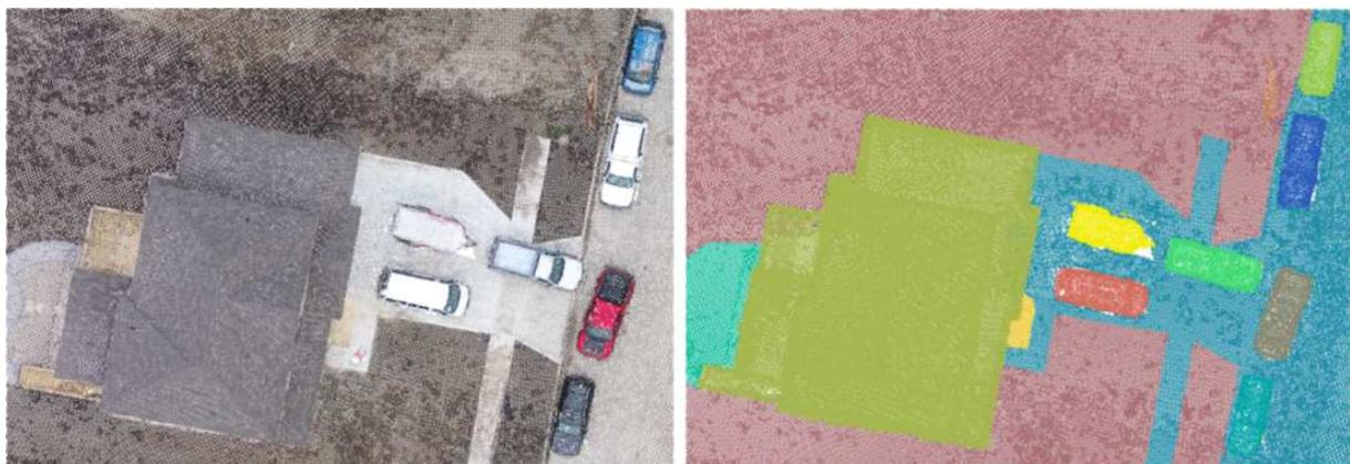
**Figure 2.11:** Extraction of individual objects. Left image shows the coloured point cloud; right image the individual objects extracted in individual colours.
