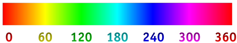
(c) Orientation encoding, in degrees, of the HSV color space.
