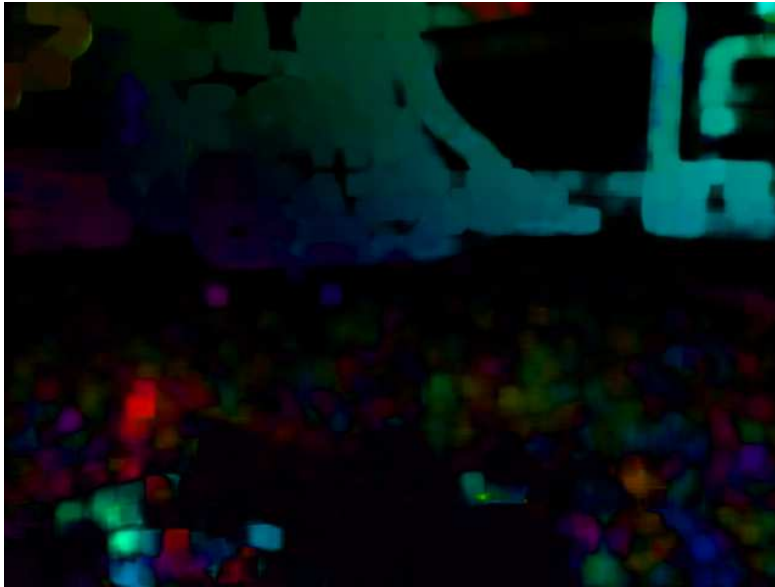
(b) Corresponding optical flow field for motion along the z axis.
