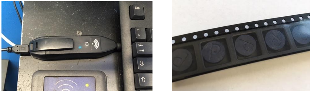
Figure 4-7: RFID tags and the RFID scanning unit
