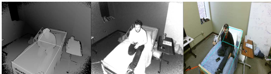
Figure 1.2: Depth, infrared and RGB image, from left to right. (Image from [19])
