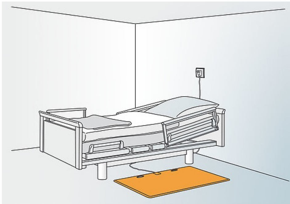
Figure 2.3: Pressure-sensitive mat in front of the bed 3 .
