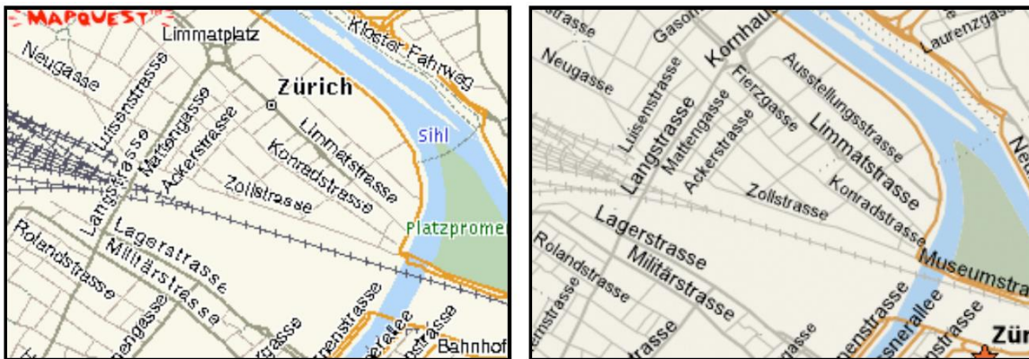
Figure 15 web map without anti-aliasing (left) and with anti-aliasing (right). Source: Jenny, Jenny and Räber, 2008
