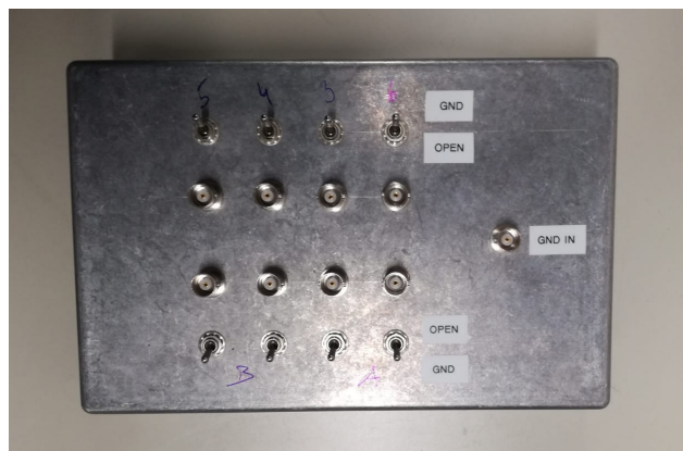
Figure 36: Photo of the switchbox, labeled the connections on top with 3 to 6 (measurement lines) and on bottom A and B for the two-channel SourceMeter to measure the temperature gradient along the NW.
