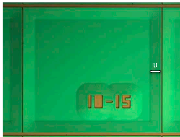
Figure 13: Mesa-pad geometry. Differential interference contrast light-microscope image of an individual mesa-pad. Showing a vertical trench width of 1\mu\text{m} , a horizontal trench width of 10\mu\text{m} and an undercut u of about 60\mu\text{m} at each pad. Taken from [60].
