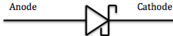
Figure 9: Electric circuit symbol of a Schottky-diode. The left side is metal which acts as the anode and the right side a semiconductor which acts as the cathode.
