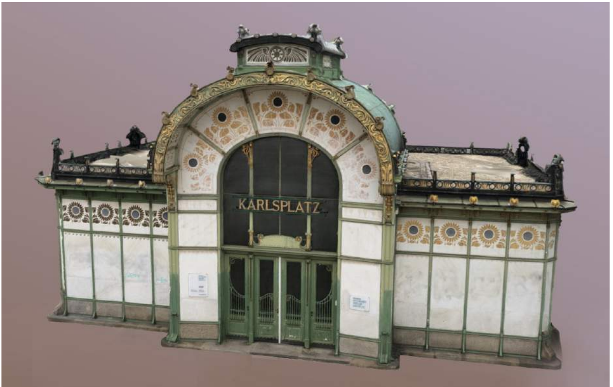
Fig.98 Final low-poly mesh with applied high resolution texture (removed graffiti from the wall).
