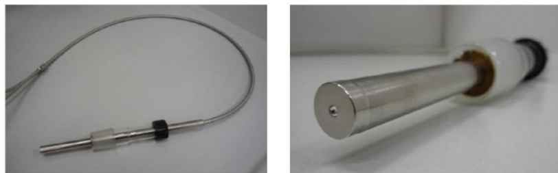
Figure 1.2.1. Mid-IR fibre and ATR probe (left) and IR probe focused on the ATR element (right).
