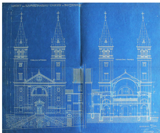
Figure 133 The Parish Church of Saint John the Baptist, Kraljeva Sutjeska: elevation view of the main façade from the south-east and cross section through the main nave viewing the bell towers in the background; segment of the second project done by Josip Vancaš, dated on 20 th April 1905 (Stari planovi crkve, Archive Kraljeva Sutjeska)
