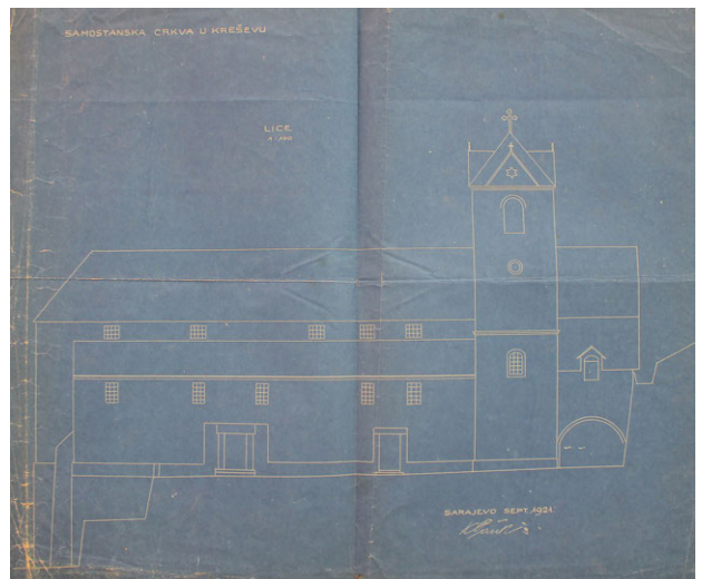
Figure A.155 The Parish Church of Assumption of Mary, Kreševo: elevation view of the eastern façade of the old church – before Pařík's intervention, segment of the project done by Karel Pařík in 1921 (Gradnja crkve i samostana, nacrti. Gr.Gr.Sp.4)
