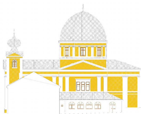
Figure 118 The Parish Church of the Holy Spirit, Fojnica: elevation view from the north, segment of the project of the current condition, done after the original project by Josip Vancaš in 1886 (Geotehnika '94, 16_18)
