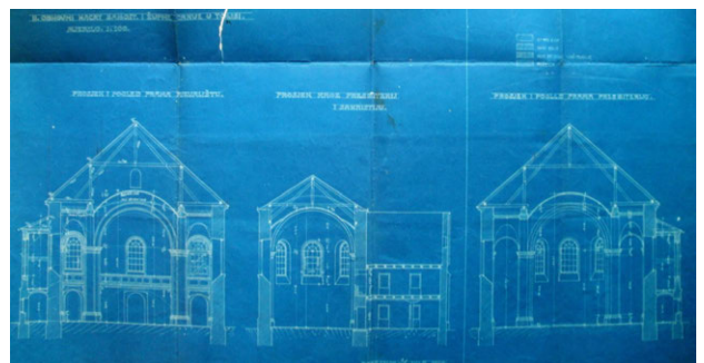
Figure A.254 The Parish Church of the Assumption of Mary, Tolisa: section views through main nave viewing the choir, presbytery and sacristy viewing the apse, and main nave viewing the apse; segment of the project „Il obnovni nacrt samostanske i župne crkve u Tolisi“ (2 nd project for reconstruction of convent and parish church in Tolisa) done by architect Josip pl. Vacaš dated on 21 st July 1910 (Archive Tolisa)
