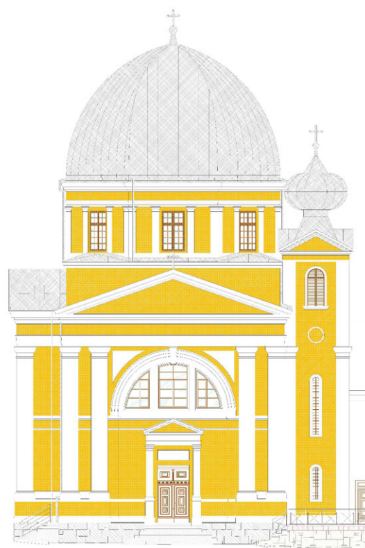
Figure 116 The Parish Church of the Holy Spirit, Fojnica: elevation view from the east, segment of the project of the current condition, done after the original project by Josip Vancaš in 1886 (Geotehnika '94, 13_18)
