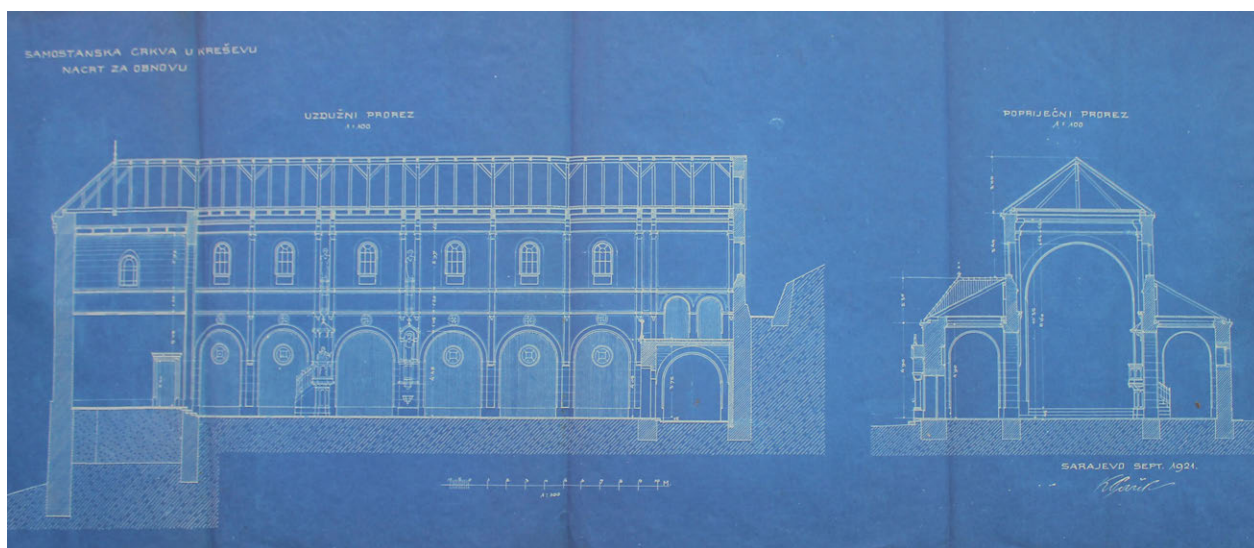
Figure A.164 The Parish Church of Assumption of Mary, Kreševo: longitudinal and cross sections through the main nave, viewing the western aisle and the apse, respectively, segment of the project done by Karel Pařík in 1921 (Gradnja crkve i samostana, nacrti. Gr.Gr.Sp.4)
