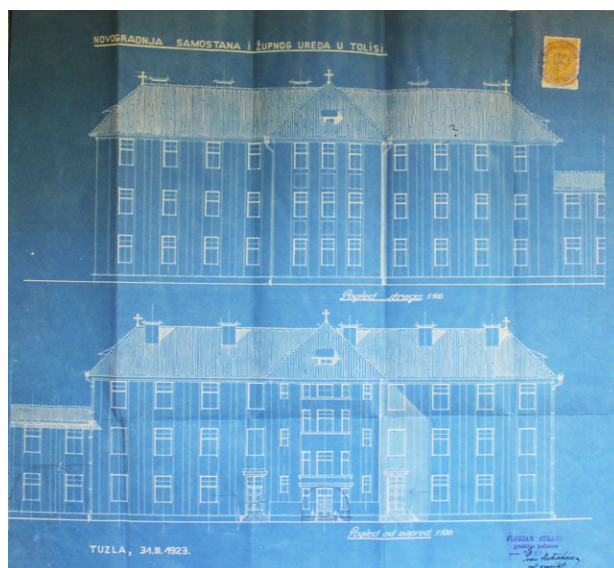
Figure A.243 The Convent of the Assumption of Mary: elevation views from south-east and north-west: garden and entrance façade, segment of the project „Novogradnja samostana i župnog ureda u Tolisi“ (New construction of convent and parish office in Tolisa) done by architect Florian Strauss, dated on 31 st March 1923 (Archive Tolisa)
