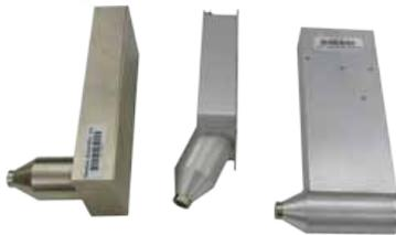
The OEM X-ray tubes are not the same as the Mini-X. The Mini-X has a USB interface to control the voltage and current through PC software. The Mini-X is an end-user, packaged device. The OEM versions are controlled by user supplied analog voltages.
