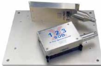
The Mini-X mounted on MP1 with X-123SDD.
