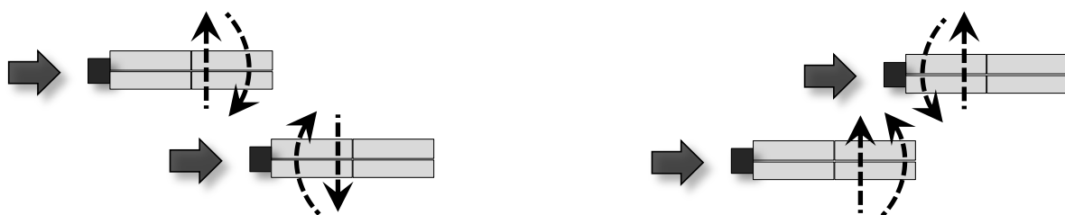
Figure 85: Force-effects occurring during an overtaking maneuver involving two pushed convoys providing the basis for the derivation of safety clearances [Tschernutter, P. 2012]
