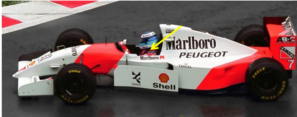
Figure 16. Huge deflector at the side of this McLaren of 1994. (Source: www.google.com . Image by unknown)
