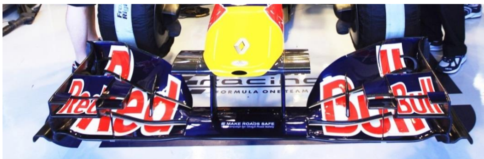
Figure 12. Front wing of the F1 car Red Bull RB7 (2011). (Source: formula1techandart.files.wordpress.com . Image by unknown)
