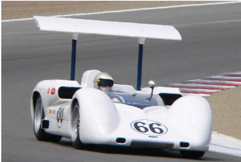
Figure 5. Chaparral 2E 1966. Here one of the first attempts to build rear wings. (Source: www.tamsoldracecarsite.net . Image by unknown)
