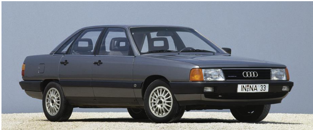
Figure 3. Audi 100 (1983) had a drag coefficient of only 0.3. (Source: www.autoevolution.com . Image by Audi)
