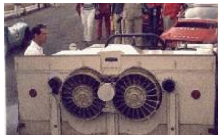
Figure 9. Big suction fans to remove the air underneath the car used by Chaparral 2J. (Source: www.formula1-dictionary.net . Image by unknown)
