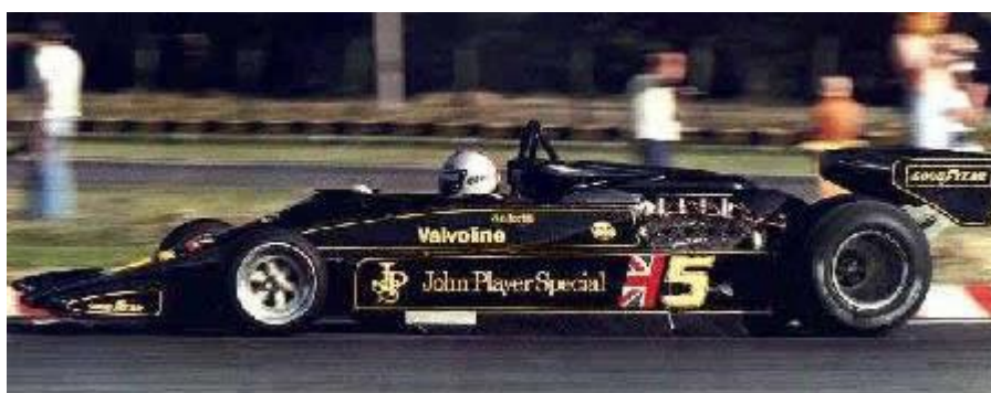
Figure 10. Mario Andretti in his Lotus (1978) with ground effect. (Source: www.formula1-dictionary.net . Image by unknown)
