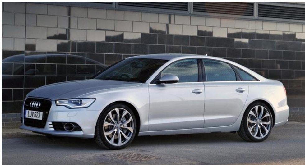
Figure 4. Audi A6 (2011-present) has a drag coefficient of only 0.26. (Source: motorburn.com . Image by Audi)
