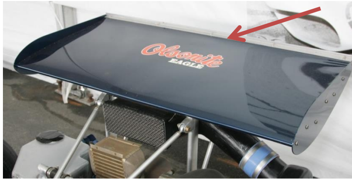
Figure 14. Gurney flap at the trailing edge of a rear wing. (Source: www.google.com . Image by unknown)
