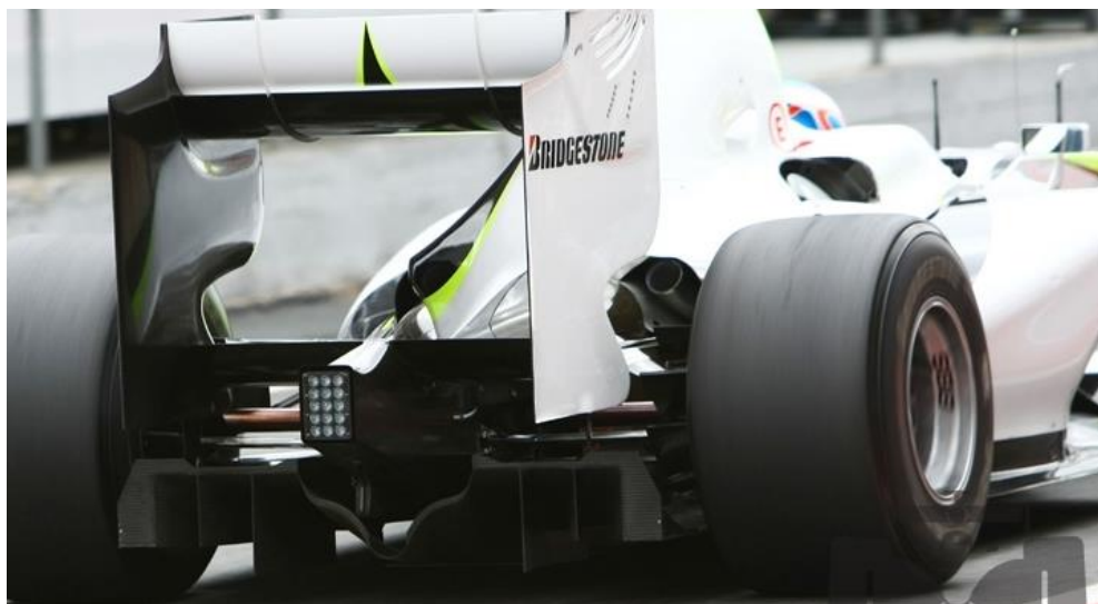
Figure 17. Double diffuser designed for Brawn GP in 2009. (Source: everythingformula1.wordpress.com . Image by unknown)
