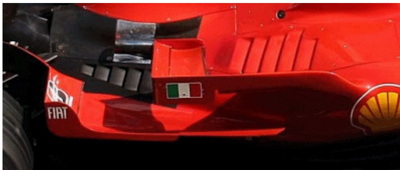
Figure 15. Detail of the body work of a Ferrari F1 where the flip-ups to guide the air over the back wheel can be seen. (Source: www.formula1-dictionary.net . Image by unknown)
