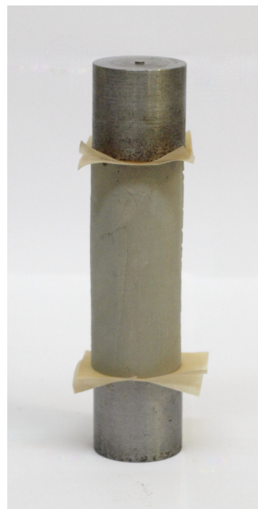
Figure 1.9: Compressive strength test setup showing steel cylinders with bottle-necks and two layers of Teflon separating them from the sample
