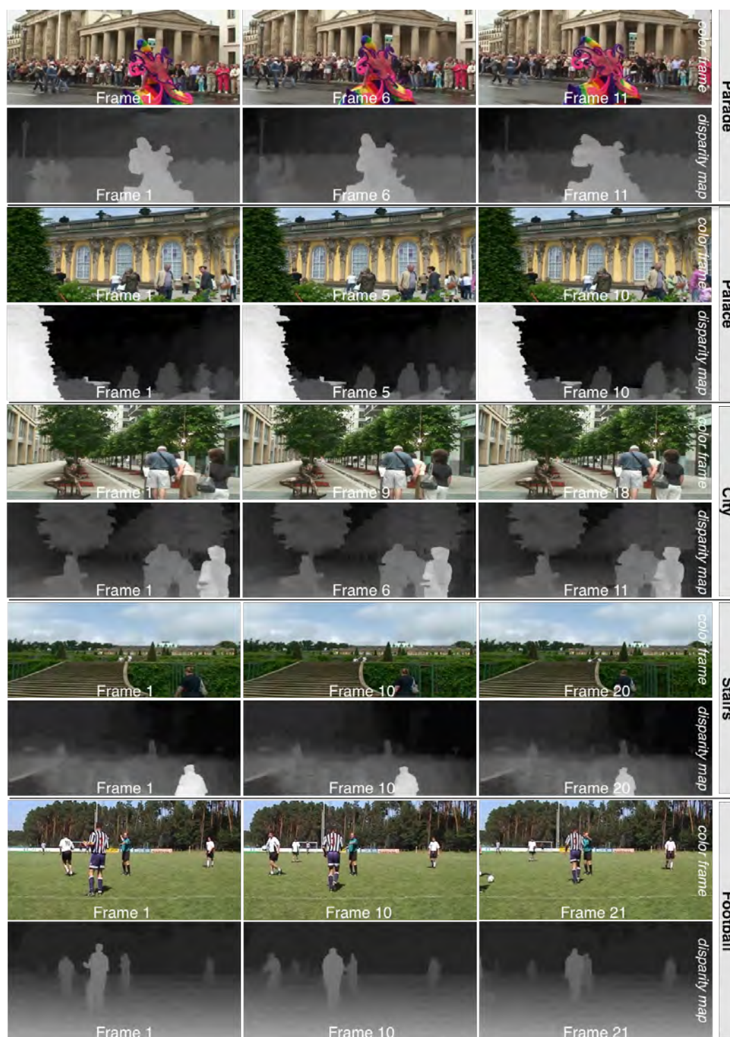
Figure A.5: Recorded stereo dataset. Color videos (left views) Parade , Palace , City , Stairs and Football (top) and reference solution (bottom). Foreground: bright , background: dark .
