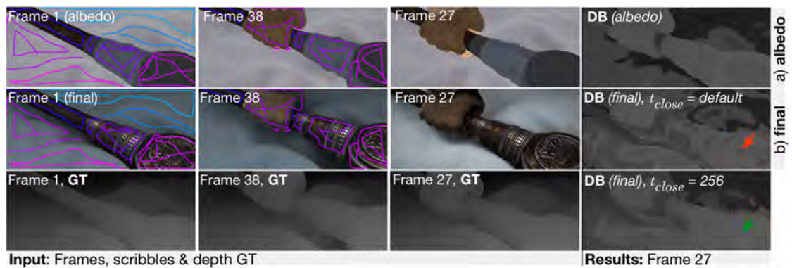
Figure 5.28: Visual evaluation of sensitivity to illumination effects. Left: Input frames with scribbles and depth GT. a) albedo rendering and b) final rendering of Ambush7 . Scribble positions and GT remain the same. Right: Our results (with DB, CON, +TC, GT OF). Newly introduced ambiguities ( red arrow ) between objects and colors that were not covered by scribbles in b) decrease the quality of our results. Adjusting t_{close} can improve ( green arrow ) the results obtained for b) . Foreground: bright , background: dark . Original videos from [27].
