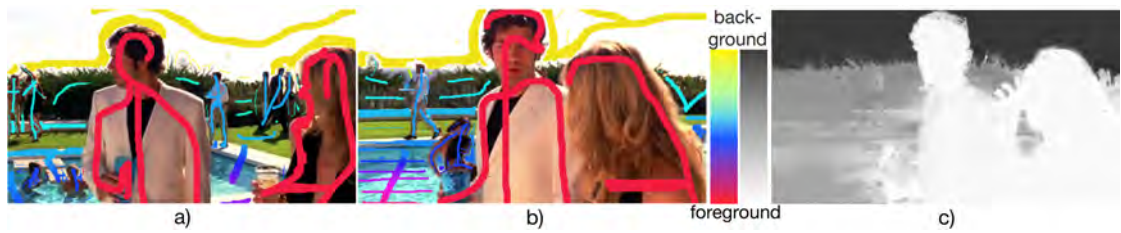
Figure 4.1: Input and output example of proposed 2D-to-3D conversion algorithm. The first frame a ) and the last frame b ) of the input video are annotated with scribbles, whose hues encode disparity. The disparity map c ) for an intermediate frame, generated by our approach, encodes disparity by gray values . Copyright of original video: Warner Bros.
