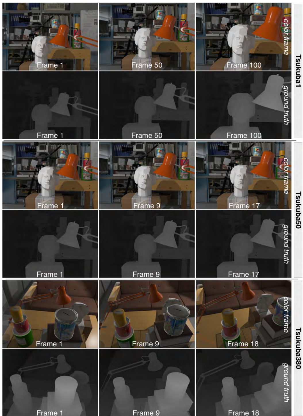
Figure A.1: Tsukuba dataset. Videos Tsukuba1 , Tsukuba50 and Tsukuba380 : Frames ( top ) and their disparity GT ( bottom ) from [102]. Foreground: bright , background: dark .
