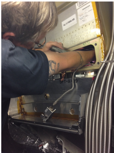
Figure 79: Connecting the warm cables to the baseplane by reaching through the pedestal.
