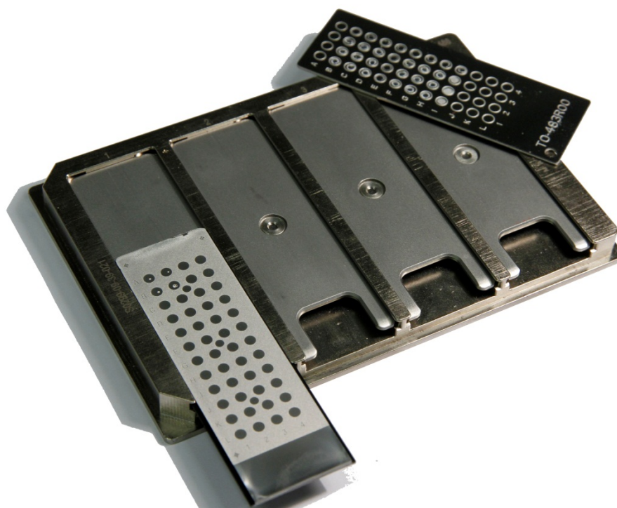
Fig.7 Target adapter with polymer target inserted; in the top right featured is a full metal target
