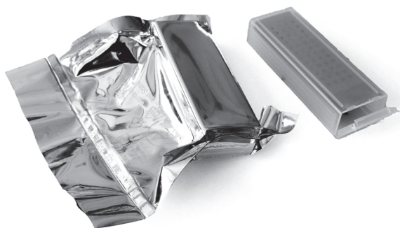
Fig. 1. MALDI MS targets stored in the container in a sealed, nitrogen-purged pouch (left) and in an open container (right) at RT.
