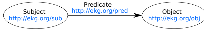
Figure 2.1: Model of an RDF Triple consisting of a subject, a connecting predicate and an object. All of them assigned to a unique label IRI.
