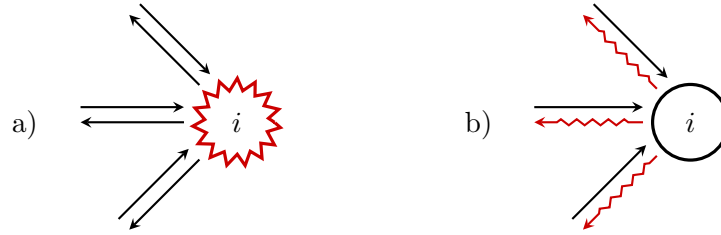
Figure 5.1: Simulation of a Byzantine-faulty agent i by a correct agent with Byzantine-faulty outgoing links. (a) The agent as a whole is considered faulty, with an a priori unclear meaning of knowledge of i . (b) We pretend that i is a correct agent, but its outgoing links behave in a Byzantine-faulty way.
