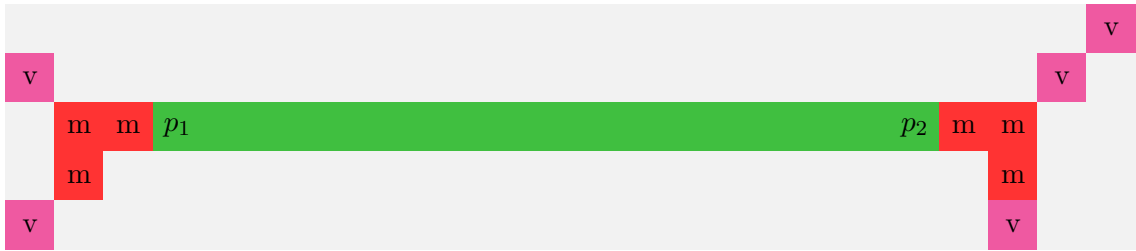
Figure 4.5: Shown in magenta the path (v); in red the margin pixels (m) of the crossing; in green the non-crossing pixels to expand; the Dijkstra expander starts in p_1 and expands until a margin pixel is found, which is not p_1 ; the algorithm will end up in p_2 and save the segment from (p_1 \rightarrow p_2)
