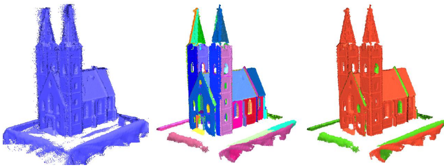
Figure 2.3: Left: the original point cloud. Center: The points that belong to a detected shape in random colors. Right: The colors are determined by type (plane = red, cylinder = green, sphere = yellow, cone = purple, torus = grey). Image by Schnabel et al. [SWK07a].
