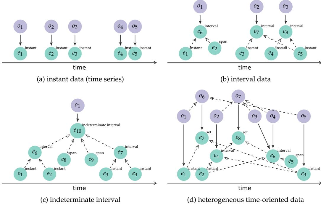
Figure 4.3.: Four temporal dataset examples depicted at the conceptual level. Each green circle  $e_x$  represents temporal element, i.e., an object of a subclass of `TemporalElement`; each violet circle  $o_x$  represents a temporal object, i.e., an object of `TemporalObject` or a subclass. Dashed lines represent composition of complex such as an interval defined by a start instant and an end instant.
