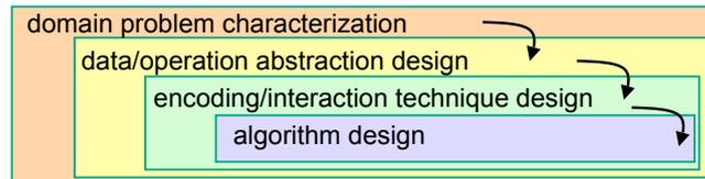
Figure 1.1.: Nested model for visualization design and validation [Munzner, 2009]
