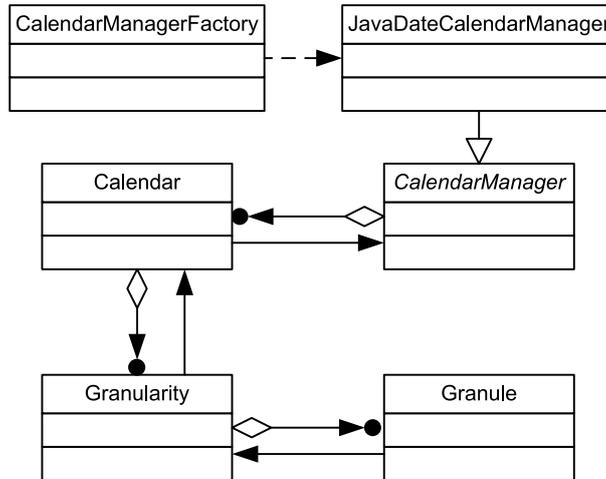
Figure 4.1.: Classes of the calendar package [Rind et al., 2013]
