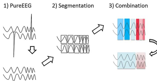
**Figure 1** The three major steps of the detection algorithm: 1) Artifact removal using the PureEEG algorithm. 2) Channel wise discharge segmentation. 3) Combination of discharge segments over several channels followed by grouping in time. The final pattern groups represent EEG patterns with multiple discharges in a certain spatial area.
