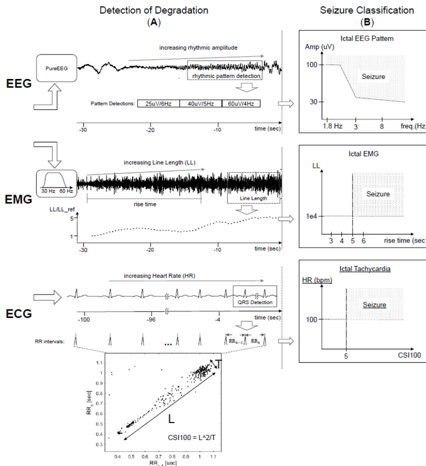
Figure 9: Multimodal seizure detection system with high sensitivity of [A5].
