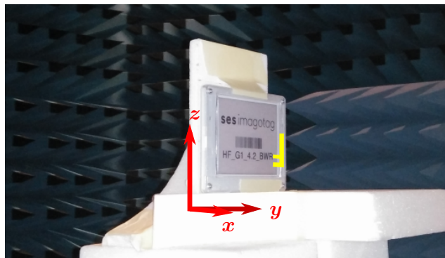
Figure 4.11: ESL as DUT mounted in the chamber. The position of the inverted-F antenna within the ESL is also indicated.
