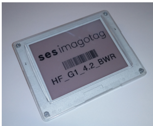
Figure 2.6: SES-IMAGOTAG electronic shelf label, as it is used in this work for \Delta RCS measurements.
