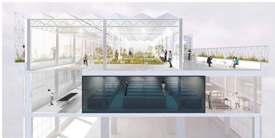
Figure 2.9: Visualization of the two levels of UF002 with hydroponic growing area on top and fish tanks below (SPACE&MATTER)
