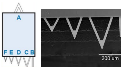
Figure 79: Cantilever layout of Bruker MSNL AFM chips. Cantilever A is located on the top of the chip and cantilevers B-F are located on the bottom of the chip 206
