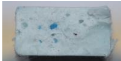
Figure 59: Fracture surface of the rBlend from tensile test
