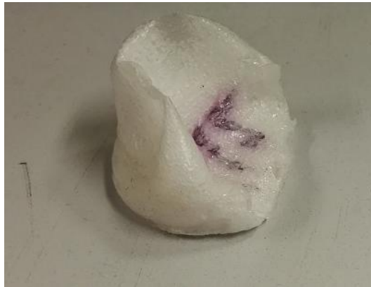
Figure 67: PP1 after foaming treatment in autoclave
