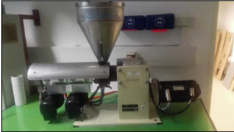
Figure 39: Extron EX-18-25-1.5 Lab Extruder
