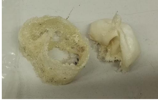
Figure 66: PP4 after foaming treatment in autoclave
