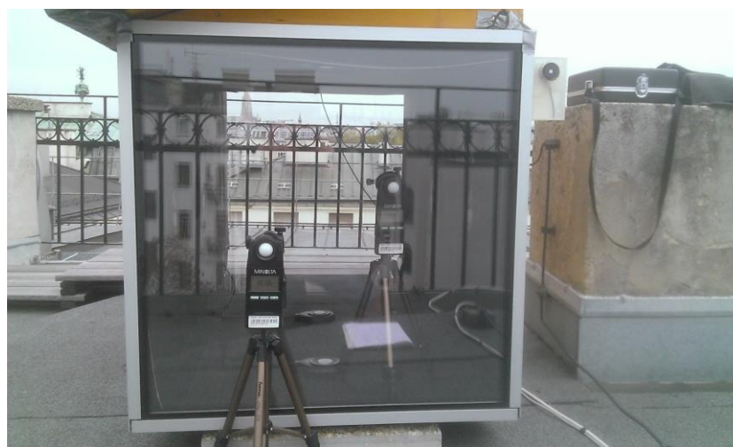
Figure 14. Image of daylight transmission measurements.
