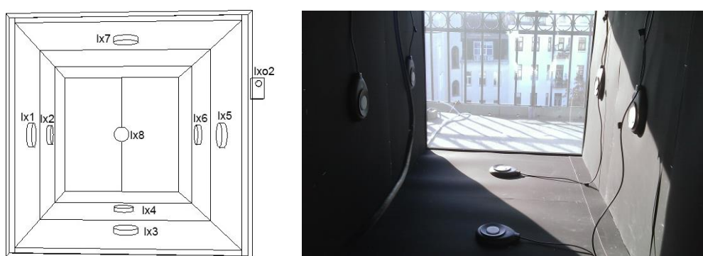
Figure 5. Left: 3D illustration of sensors distribution. Right: Image of sensors inside the test bed.
