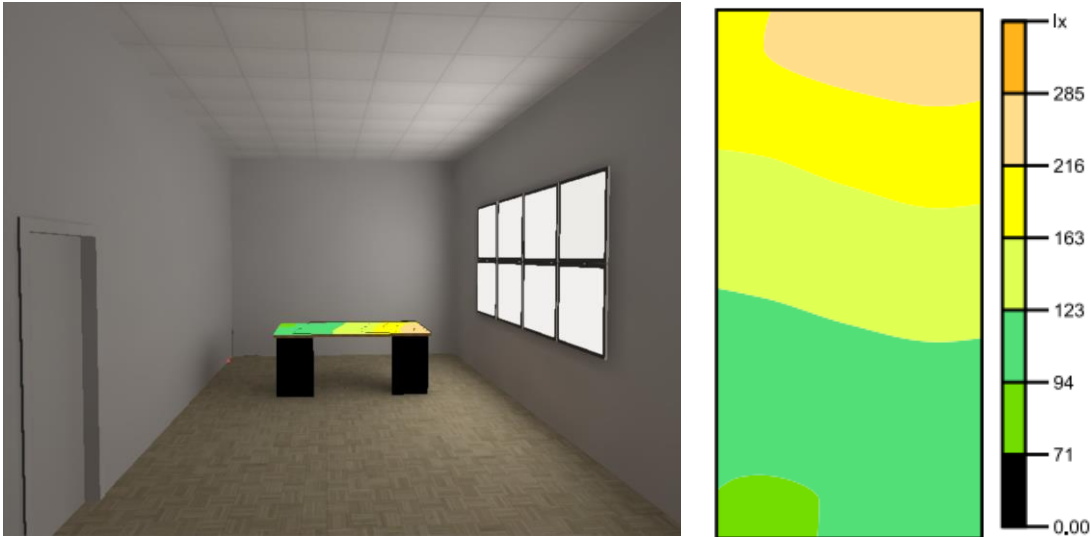
Figure 38 . Artificial light illuminance on task area
