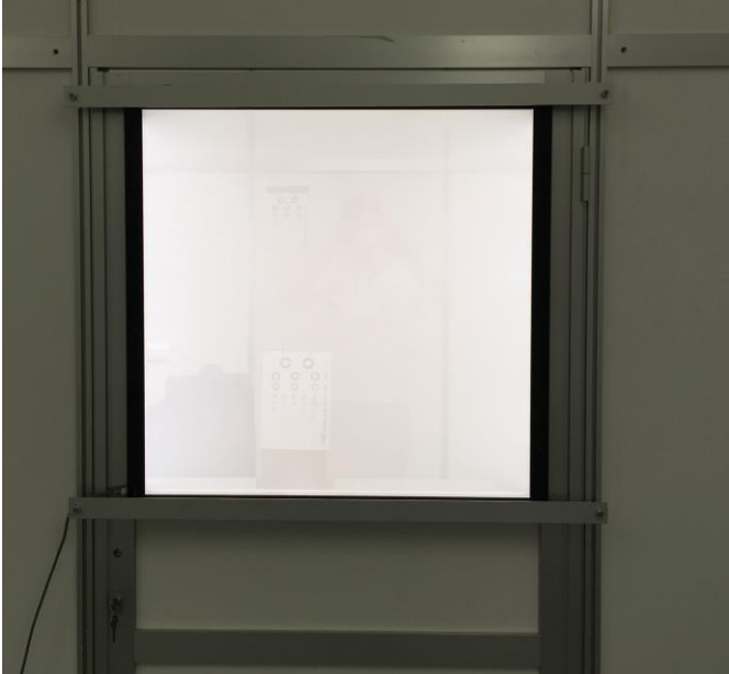
Figure 44. Image of acuity test at 1m viewer distance
