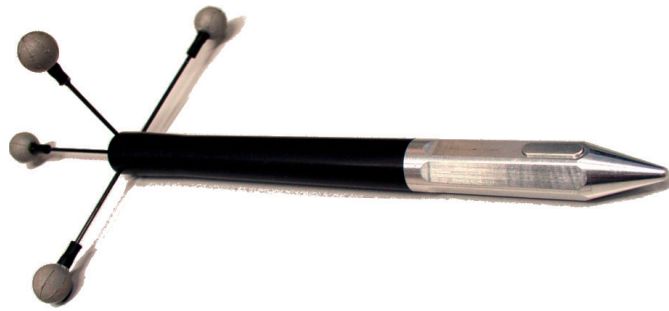
Figure 2.2: A trackable wireless, one-button pen with retro-reflective markers [22].
