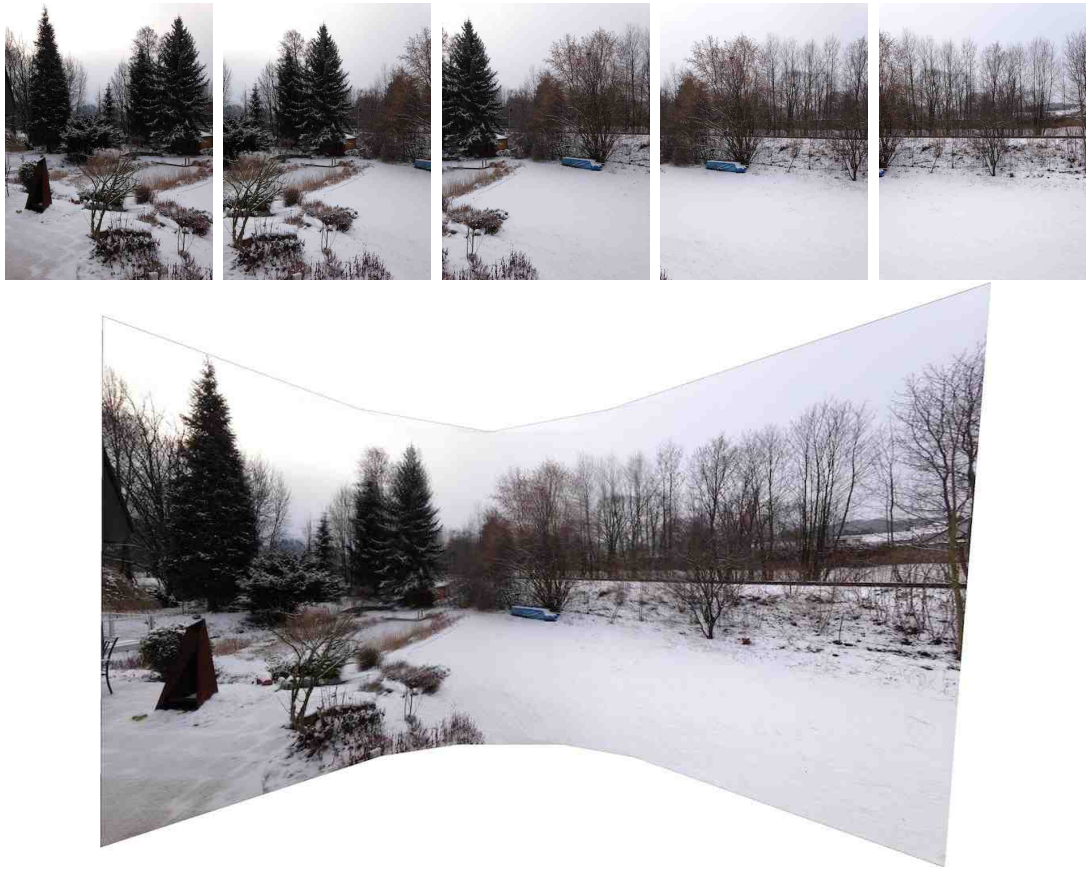
Figure 3.1: Example of Image Stitching. The top row of images are separate images of a panorama, they are registered to each other, transformed and blended into a single panorama (bottom image).
