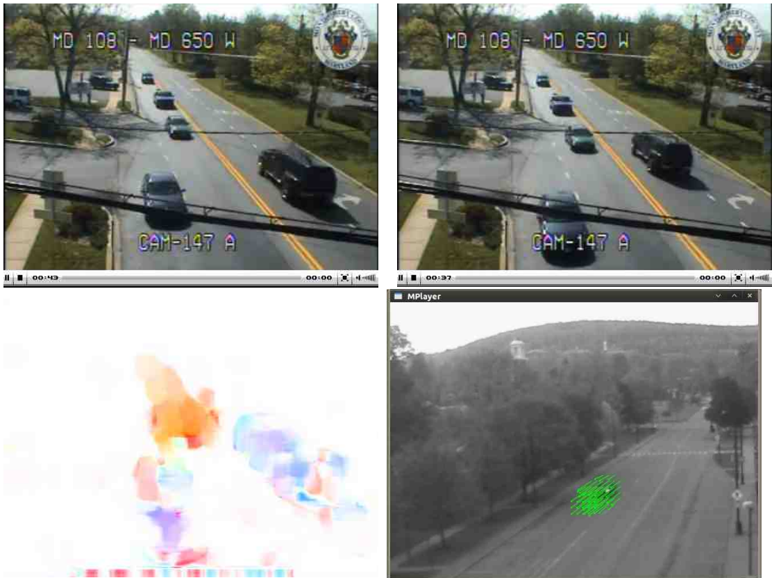
Figure 3.14: Examples of Optical Flow. The top left and right image are two consecutive frames of a video with moving cars. The bottom left image shows the optical flow with color coded movement directions. The bottom right image shows a similar scene where the optical flow is visualized with vectors.
