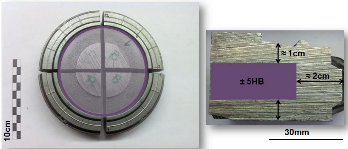
Fig. 3.3: Region of trust chosen taking into account the Brinell hardness maps.
