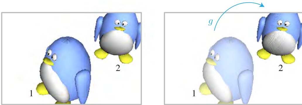
Figure 1.2: Brightness constancy assumption. The tendency of the assumption of brightness constancy to break down as displacements become large is especially easy to see in the presence of rotation, whether due to rotational motion of the scene relative to the camera or—unless the scene is genuinely Lambertian [Ang06], whereby shading is invariant to the pose of the camera—to that of the camera relative to the scene. Intuitively, differences in shading are due to the further penguin being illuminated frontally, while the closer one is illuminated from the side (figure best viewed in the electronic version of this thesis).
