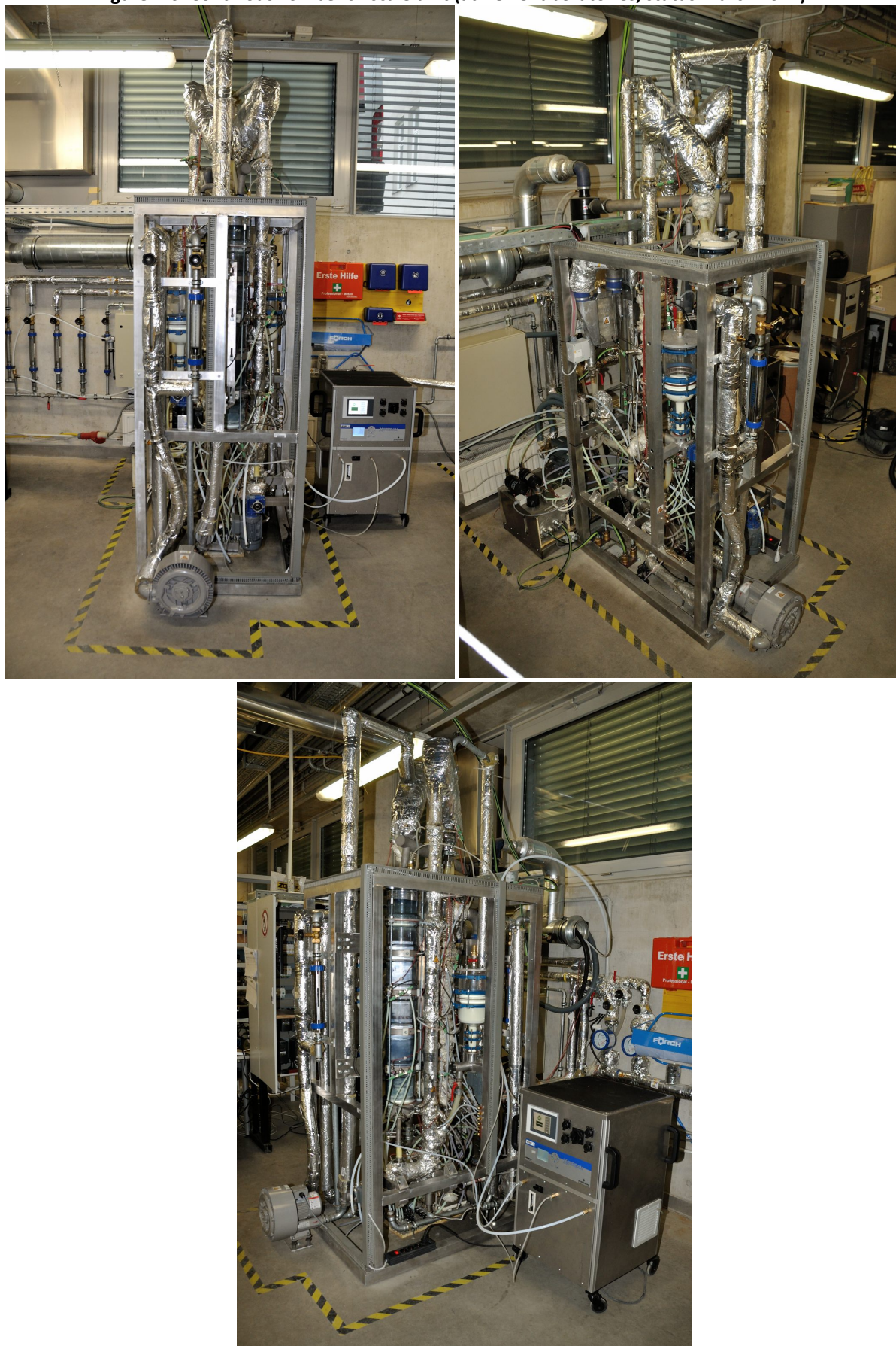
Figure A 6: Continuous TSA bench scale unit (at BOKU laboratories, status March 2014).
