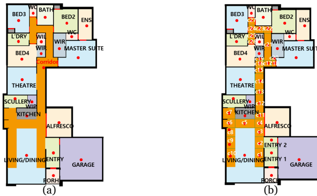
Figure 4. Topologically and semantically defined space (a) semantically defined subspaces.; (b) divided connection space
