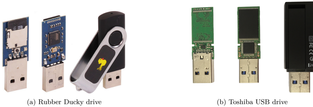
Figure 5.2: A Rubber Ducky USB drive featuring an additional 128 MB SD card (left) and a Toshiba USB drive featuring a Phison PS2251-03 chip (right)
