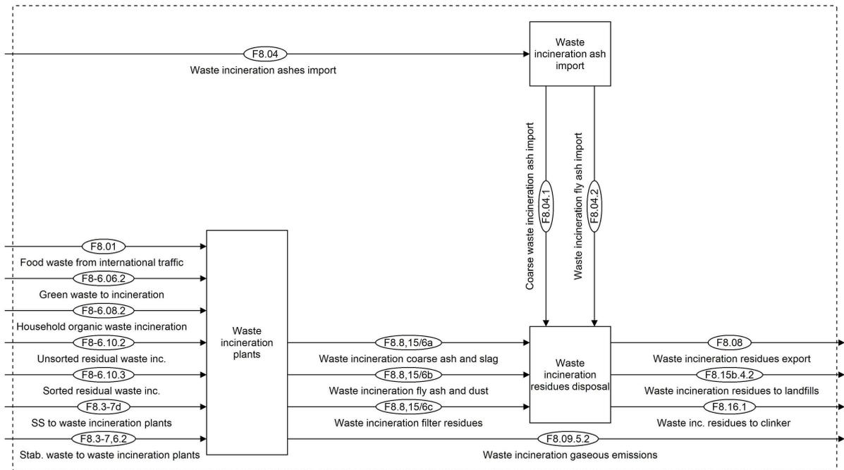
**Fig. A.31:** MFA structure of the Austrian P-N system 2015 - Subsubsystem *Waste incineration*.
