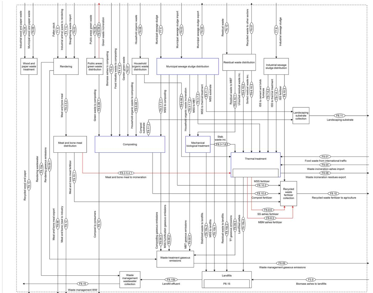
**Fig. A.43:** MFA structure of the Austrian P-N system 2015 - Subsystem *Waste management*. Changes to the original model structure under the Combined measures scenario. Changes to the original model structure are marked in red.
