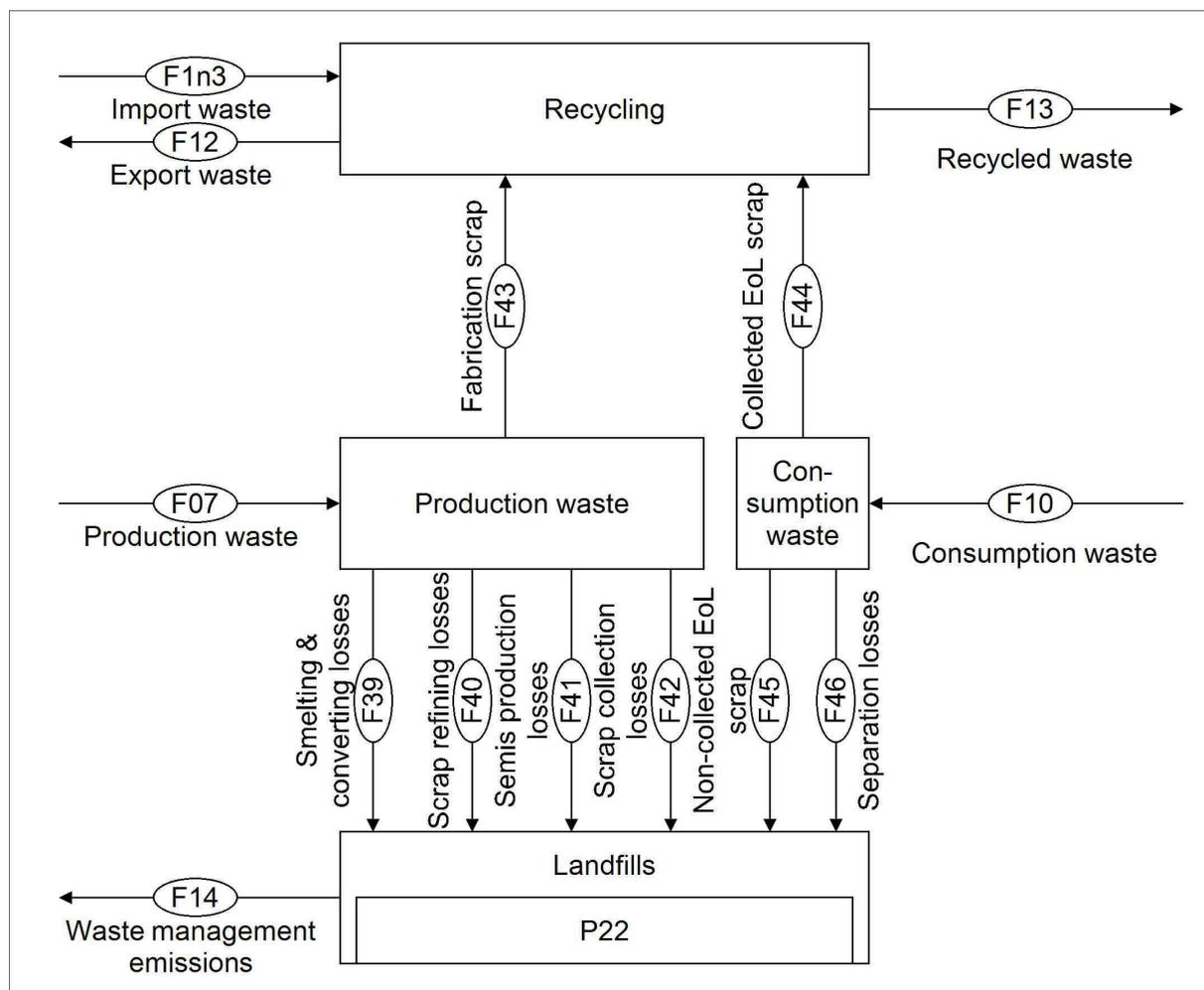
**Fig. A.51:** MFA structure of the EU 28 copper system 2014 in the multi-level generic framework - Subsystem *Waste management*.
