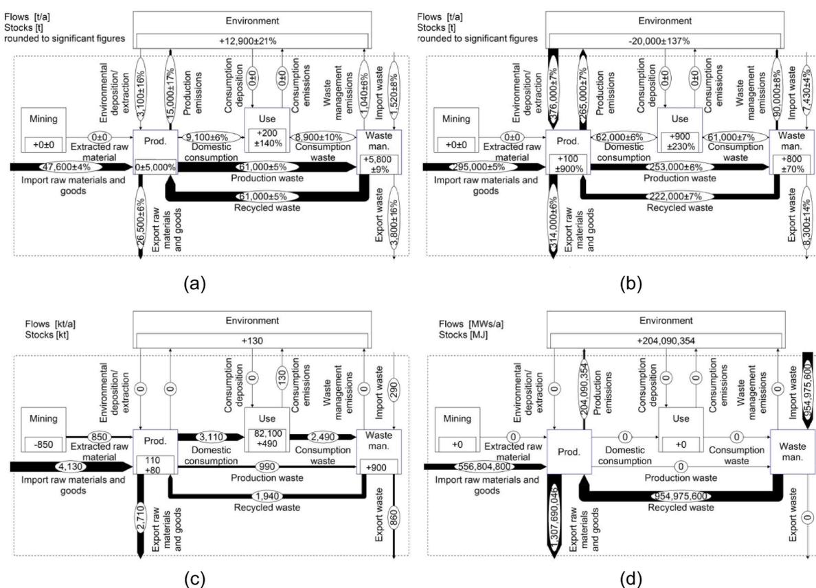
**Fig. 4.5:** Generic MFA system of the three case studies: (a) Austrian P-N system-P; (b) Austrian P-N system-N; (c) EU28 copper system; (d) Energy flows in Karlskoga heat and power plant.
