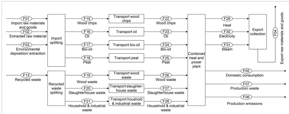
Fig. A.52: MFA structure of the Karlskoga combined heat and power plant 2016 in the multi-level generic framework - Subsystem *Production*.
