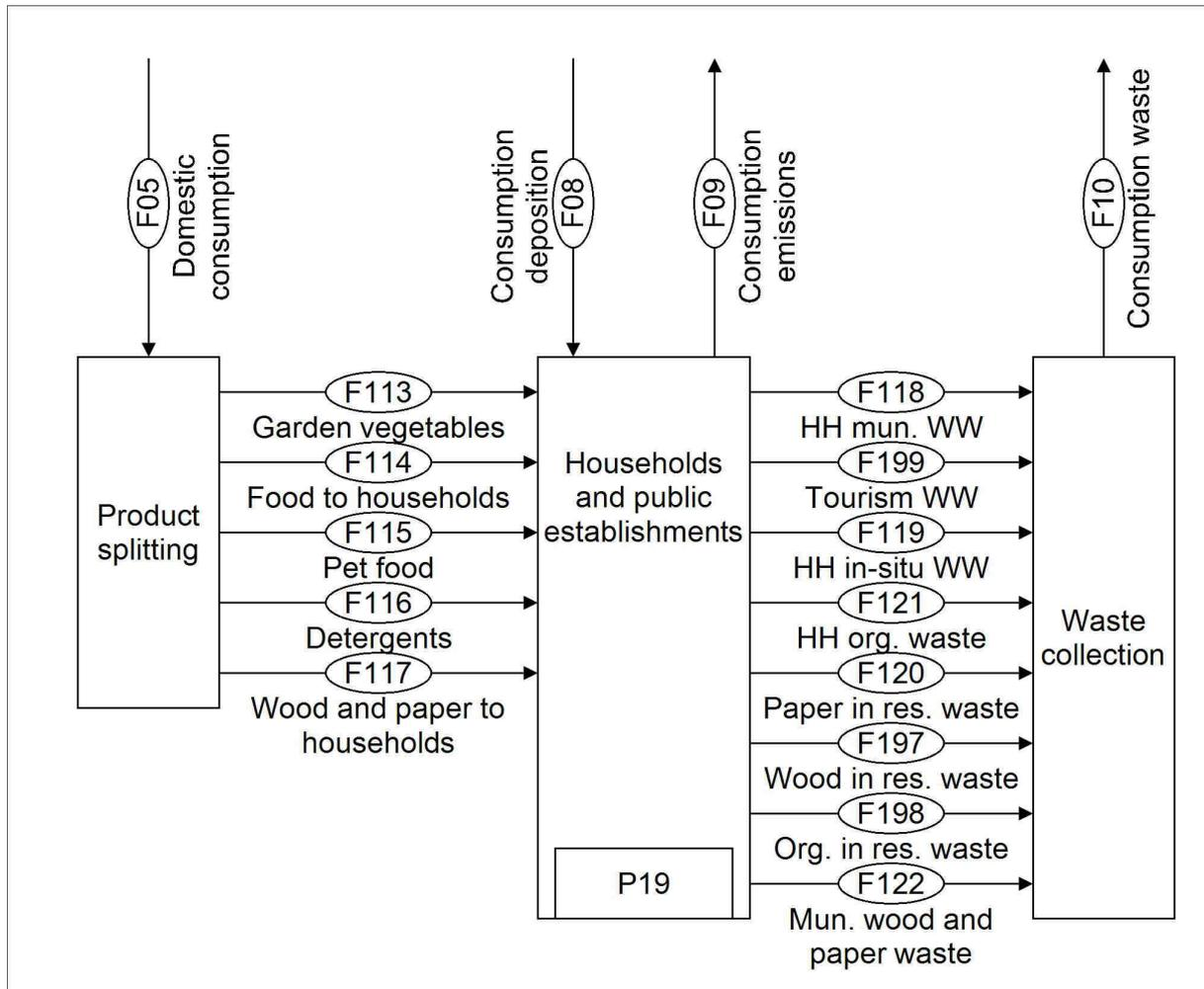
**Fig. A.48:** MFA structure of the Austrian P-N system 2015 in the multi-level generic framework
