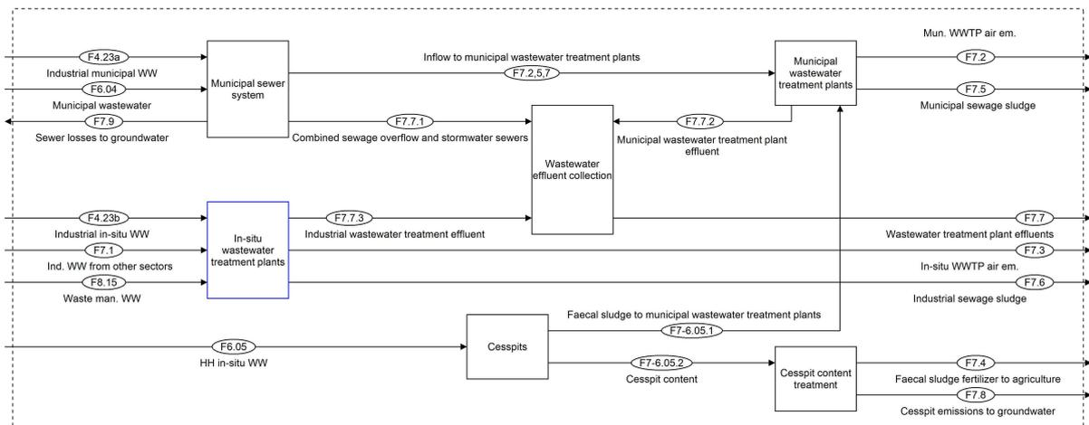
Fig. A.24: MFA structure of the Austrian P-N system 2015 - Subsystem *Wastewater treatment*.
