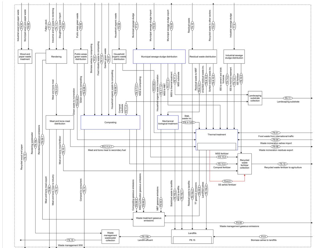
**Fig. A.42:** MFA structure of the Austrian P-N system 2015 - Subsystem *Waste management*. Changes to the original model structure under the measure *Increased P-recovery from sewage sludge*. Changes to the original model structure are marked in red.
