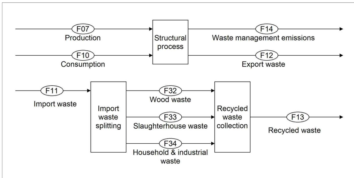
Fig. A.53: MFA structure of the Karlskoga combined heat and power plant 2016 in the multi-level generic framework - Subsystem *Waste management*.
