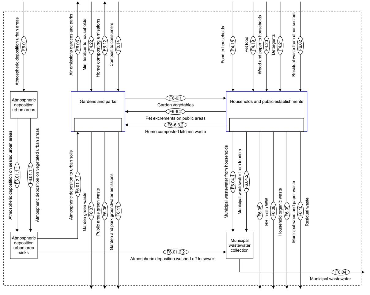
Fig. A.20: MFA structure of the Austrian P-N system 2015 - Subsystem *Households and public establishments*.
