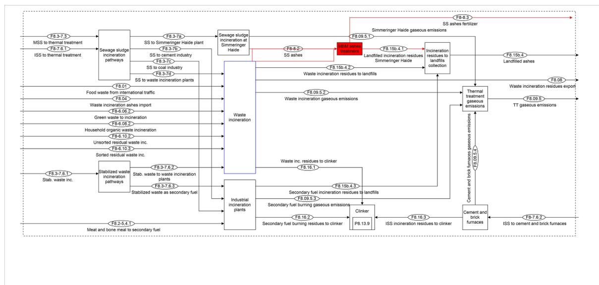
**Fig. A.45:** MFA structure of the Austrian P-N system 2015 - Subsystem *Thermal treatment*. Changes to the original model structure under the measure *Increased P-recovery from sewage sludge*. Changes to the original model structure are marked in red.
