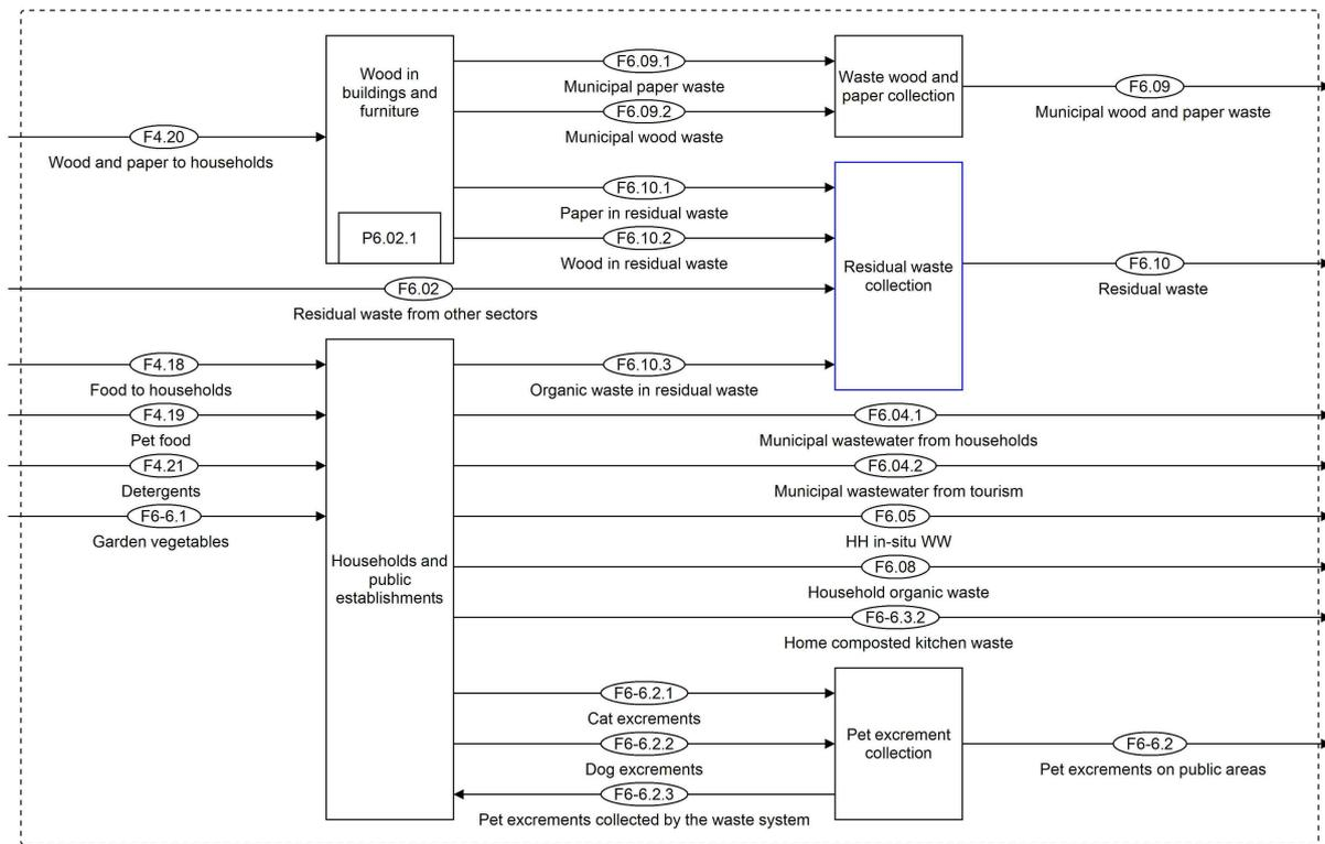
Fig. A.22: MFA structure of the Austrian P-N system 2015 - Subsystem *Households and public establishments*.
