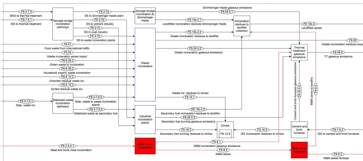
**Fig. A.44:** MFA structure of the Austrian P-N system 2015 - Subsystem *Thermal treatment*. Changes to the original model structure under the measure *Increased nutrient recovery from meat and bone meal*. Changes to the original model structure are marked in red.
