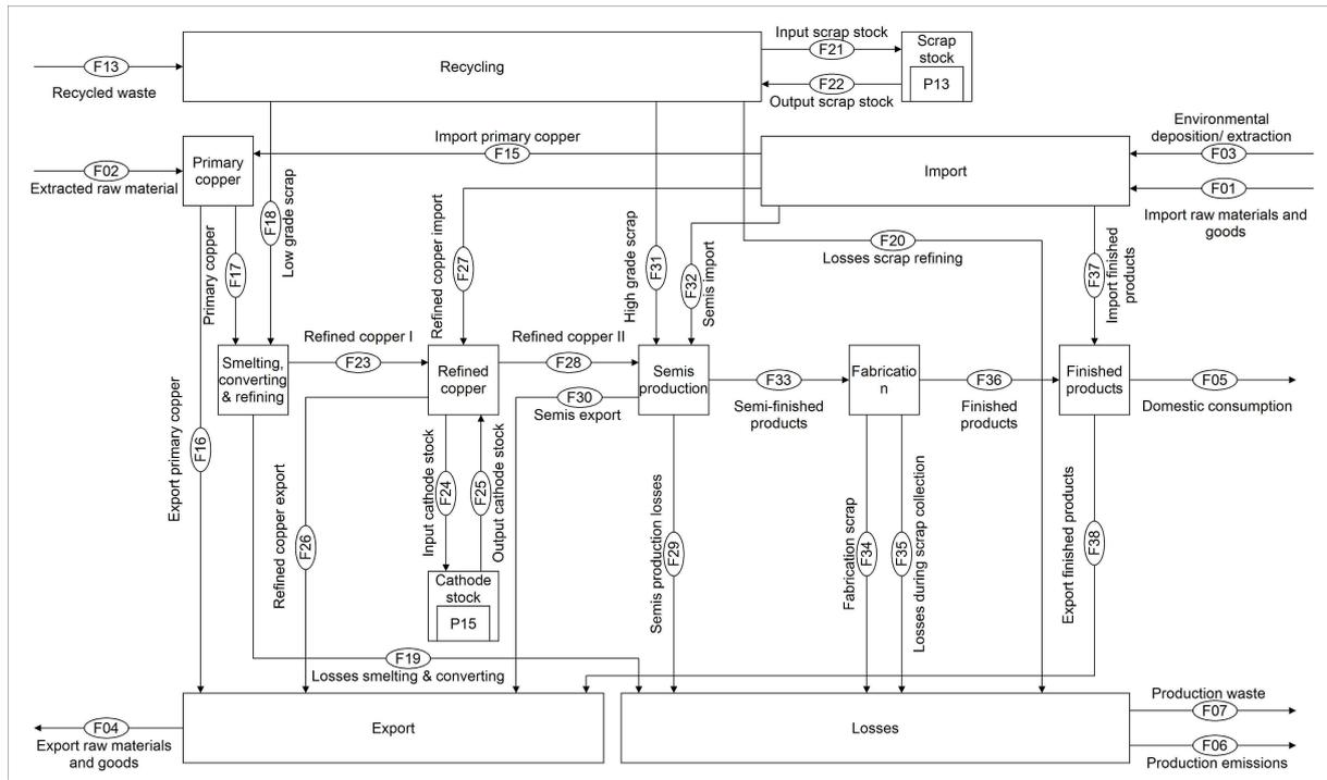
**Fig. A.50:** MFA structure of the EU 28 copper system 2014 in the multi-level generic framework - Subsystem *Production*.
