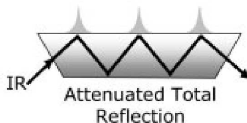
Figure 2.23.: Illustration of the ATR technique (adapted from [64])
