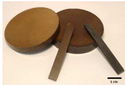
Figure 11: P84/PPPI composite, hot compression moulding samples and cut out test specimens
