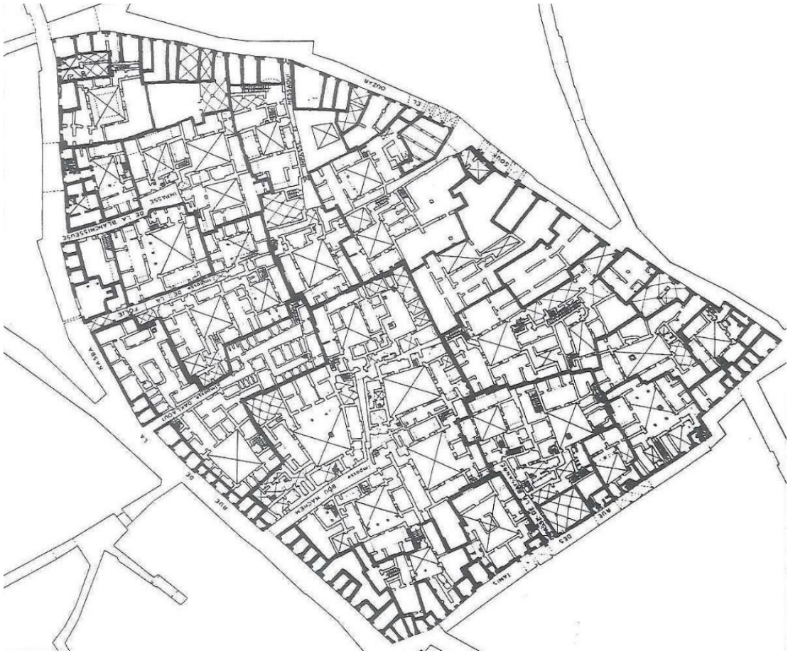
Fig. 2.2.1.1 Beijing 1750 – Detail of the Complete Map of the Capital City during the Qianlong Era, showing deep territoriality with main streets and gated side streets and sequences of several courtyards (Habraken 1998)
