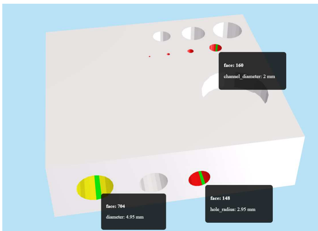
Figure 4.6: Annotated testobject with different holes (orientation, shape)
