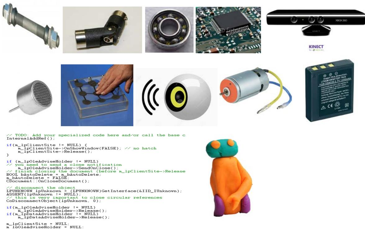
Figure 3.7 Robot parts (left to right top down): kink, hinge, bearing, micro controller, 3D camera, microphone, touch sensor, speaker, motor, battery, software, and hull.
