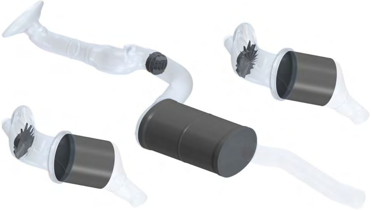
Figure 4.6: CFD domains for the simulation of UWS preparation: underbody type (centre) and close-coupled type SCR system with mixer 1 (top right) and mixer 2 (bottom left). The systems not to scale, mixers and SCR catalysts are shown in grey.
