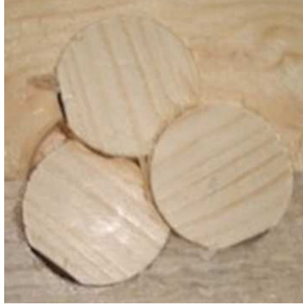
Figure 3.1: Defect covered by three patches.
