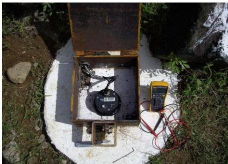
Figure 24 Digital accelerograph (Mateo 2009) Figure 25 Analogue accelerograph (Dadisp 2014)
