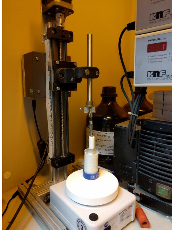
Figure 9: Dip coating setup
