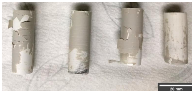
Figure 23: Delamination of intermediate layers after pyrolysis
