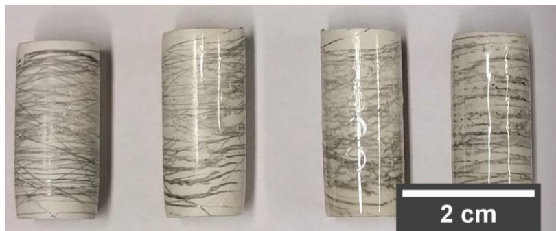
Figure 10: Samples that were marked and then masked. Excess PS is still present.
