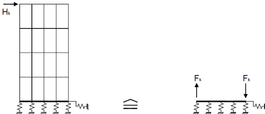
Figure 3.9: Horizontal load equivalence with a pair of loads operating in opposite directions [47].
