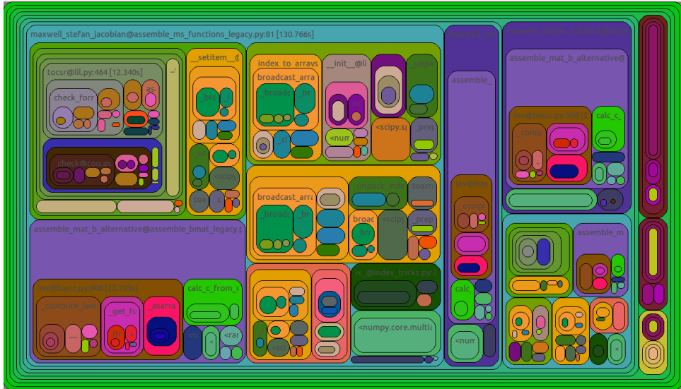
Figure 4: Graphical output of RunSnakeRun processing profiling data collected by cProfile. The block for the Maxwell-Stefan jacobian assembly is taking up over 75% of the runtime. This data was collected by performing 10 timesteps of the Duncan-Toor experiment, cf. section 5.2.
